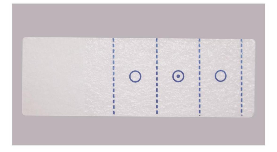
The subarea location of the slide ensures that the minimum reagent quantity exerts its maximum effect. 1–3 tissues can be dyed simultaneously.
