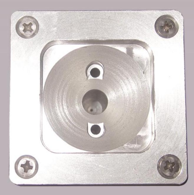
The clean-out opening of the drop tube can clean both the interior and exterior walls of the drop tube and avoid cross-contamination.
