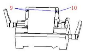
If a high-profile blade is needed, use a 3mm hex wrench to remove the four bolts (7), detach the anti-curling plate (8), and then unscrew the two screws (9) on the spacer (10) and remove the spacer (10). After installing the blade, reattach the anti-curling plate (8) and secure it with the four bolts (7).
