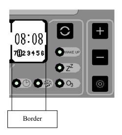
Press and the border of the time display area will be bolded. When the light is on, It enters sleep time mode as the left diagram illustrates. Press to enter wakeup time setting. The value can be set through Press to switch to minute setting, then press again to switch to day setting. Users can individually set the wake-up time for Monday through Sunday.
