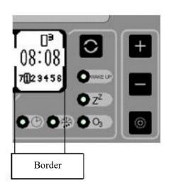
Press and the border of the time display area will be bolded. When the light on, it enters disinfection time mode as the left diagram illustrates. Press to enter disinfection time setting. The value can be set through Press to switch to minute setting, then press again to switch to day setting. After completion, press to enter sleep time setting or it will automatically exit after 5 seconds of inactivity.
