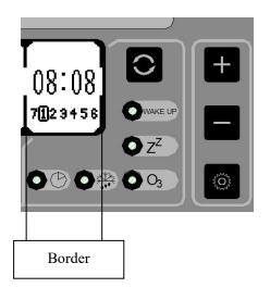
Press , and the border of the time display area will be bolded. When the light on, it enters real-time mode as the left diagram illustrates. Press to enter real-time clock setting. The value can be set through ress to switch to minute setting, then press again to switch to day setting. After completion, press to enter defrost time setting or it will automatically exit after 5 seconds of inactivity.
