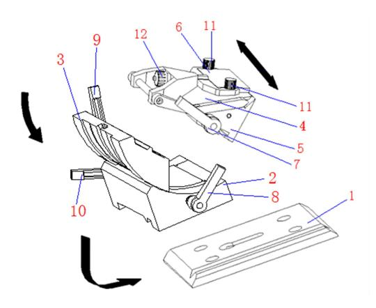
As shown in the diagram, the blade holder consists of the following components: base (1), vertical slider (2), rotating slider (3), movable knife clamp (4), fixed knife clamp (5), anti-curling plate (6), lever 1 (7), lever 2 (8), lever 3 (9), lever 4 (10), anti-curling plate locking knob (11), anti-curling plate height adjustment knob (12).
