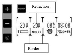
Press **RETRA**, the border will be bolded, then press to enter retraction setting. The value can be set by **H**. After completion, press again to exit or it will automatically exit after 5 seconds of inactivity.
