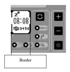
Press and the border of the time display area will be bolded. When the light on, it enters sleep time mode as the left diagram illustrates. press to enter sleep time setting. The value can be set through ress to switch to minute setting, then press again to switch to day setting. After completion, press to enter wake up time setting, or it will automatically exit after 5 seconds of inactivity.
