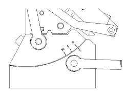
At this point, the blade holder itself and its attachment to the machine base can be secured by using the four fixed rods. Before tightening, you can adjust the positions, such as front-back, left-right, and rotational angles, as needed.
