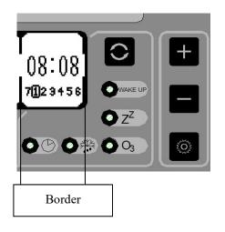
Press and the border of the time display area will be bolded. When the light is on, it enters defrost time mode as the left diagram illustrates. Press to enter defrost time setting. The value can be set through Press to switch to minute setting, then press again to switch to day setting. After completion, press to enter disinfection time setting or it will automatically exit after 5 seconds of inactivity.
