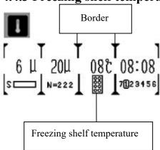
After pressing , as shown in the left diagram, the border of the temperature area will be bolded. When the display shows , it entered freezing shelf temperature display mode. The temperature on the display reflects the actual temperature of the freezing shelf.
