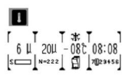
Press and hold for a few seconds to turn on/off specimen clamp peltier function. When the function is activated, ""
