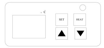
SET--- This function is used to set the temperature. Press the button, and the indicator lamp will illuminate, displaying the set temperature value on the LED screen. Adjust the temperature using
