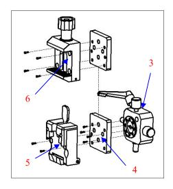
There are two types of clamps: C-type specimen clamp (6) and Quick release cassette clamp (5).
