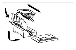
As shown, each knife holder component is detachable for separate cleaning. The slide rails, locking lever, blade clamp, and connecting parts are susceptible to contamination. It's particularly crucial to clean the blade clamp before each installation to prevent compromised blade tightness and ensure high-quality sections.
