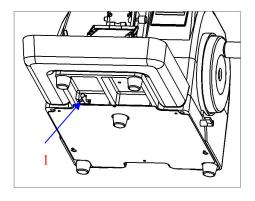
The equipment's balance, regulated by an internal spring connected to the wheel, can be affected by changes in temperature, humidity, and long-term stress on the spring, leading to an imbalance in rotation. To address this issue, lift the bottom of the equipment and rotate the nut (1) as shown in the diagram.
