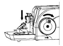
• Once the above steps have been completed, check and ensure that all locking levers on the knife holder, on the base and on the specimen clamping system have been tightened. Lastly, unlock the right handwheel to trim.
