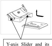
Y-axis Slider and its corresponding lever
