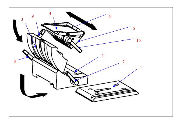
As the diagram shows, the knife holder is composed of the following parts: Z axis slider (1), Y axis slider (2), X axis slider (3), clamp 2 (4), clamp 1 (5), knife guard (6), lever 2 (7), lever 2 (8), lever 2 (9), lever 1 (10).
